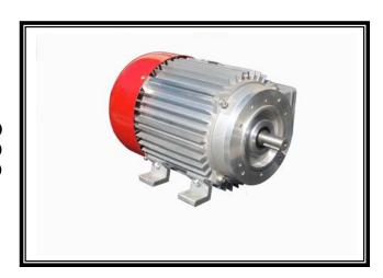
Completely Sealed AC Generatpr AVR controlled Voltage Voltage Accuracy +\_1 % Motor Starting 300 % Galvanized Aluminum Housing High Speed coating (6000 RPM) Overall Efficiency 86 % Operating Speed 3600 RPM
