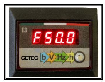
With the push of a Button You instantly can see AC Voltage DC Voltage Frequency Running Hours Total Hours
